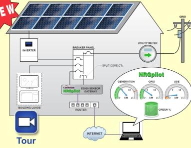
Simple installation using split core clamp on CTs supplied for 120/240 breaker panels
